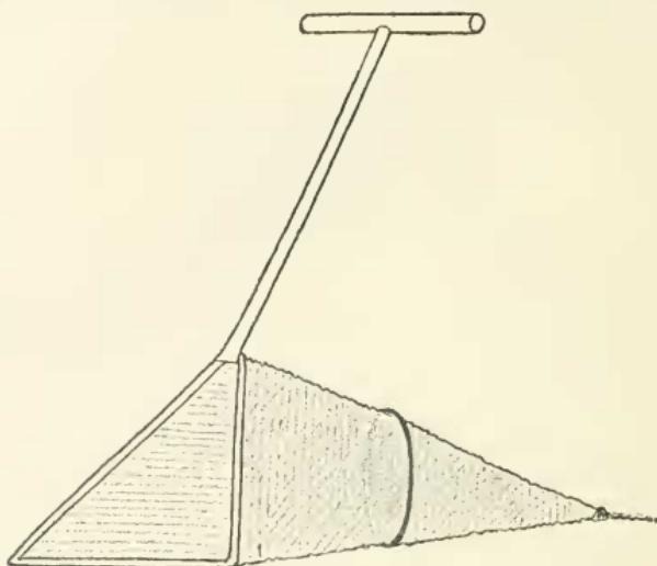
nets are of horsehair cloth, as used for sieves, but ordinary linen cheese-cloth is mostly used. At about 18 inches from the pocket of the net a cane ring with netting of about three quarters of an inch mesh is inserted across it, so as to prevent the entrance of larger objects (crabs, shrimps, &c.) among the Mysids.
